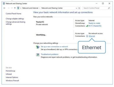
B. Go to "Properties"  $\rightarrow$  "Internet Protocol Version 4(TCP/IPv4)", select "Obtain an IP address automatically" or "Use the following IP address", then assign a static IP manually within the same subnet of the device.
